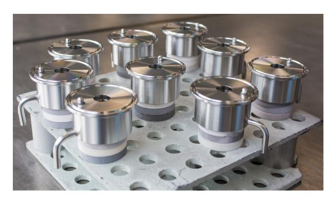
We use our own tools for this or special positioning tools. Alternatively, it could be decided to join the materials by tack welding so that they remain in the right place during the brazing process without using a positioning tool. The engineer will determine the parameters for tack welding in advance, so that it does not affect the desired end result.
