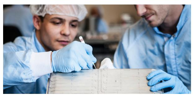
A solder assembly in which a heating wire is vacuum soldered to a product.
